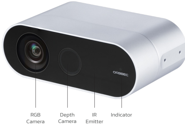
Femto Bolt front view showing components
